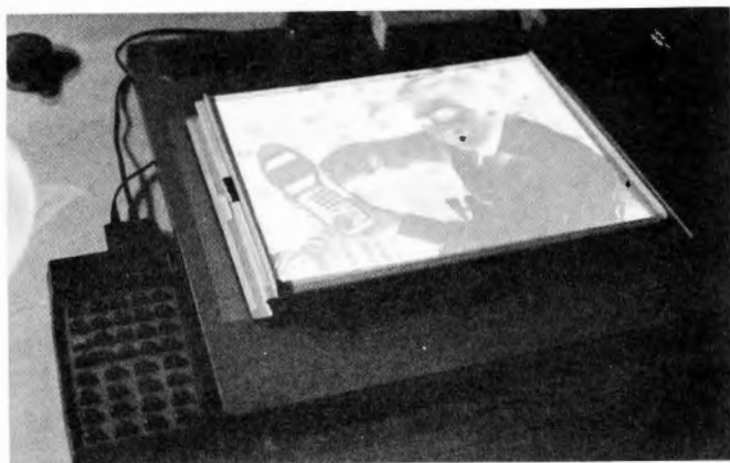
Step 3 With paper in the easel and filter in place, press AUTO to automatically expose for the recommended time.
