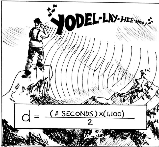
If an object is only five feet away, the echo returns in 9 milliseconds. A 71 using HP-IL, or even a 41 using the Time Module pads described in Chapter 3, isn't nearly fast enough to detect this echo. Assembly language routines using the CPU lines, however, have absolutely no problem.
