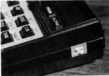
A DIP switch on the 41's exterior can temporarily disable the internal time module while the versatile adapter is plugged in. The module can be made "invisible" without the loss of time, date or accuracy factor.
