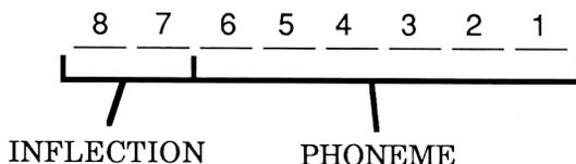
The two most significant bits determine the pitch, or inflection, at which the phoneme is spoken. The greater the inflection bits, the higher the pitch. Therefore, if you wish to increase the pitch of any phoneme, simply add multiples of 64 to the phoneme's address. For example, to hear it sing "A" in 4 musical keys:
