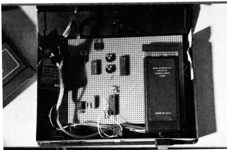
Inside the controller is an IL Converter and a small, unregulated power supply. A 5v regulator was added to protect the circuitry. The front panel (bottom) contains the IL receptacle, 3-pin miniature phone jack for the RAT, and a master power switch. The enlarger plugs into an AC receptacle mounted on top of the case (not shown).
