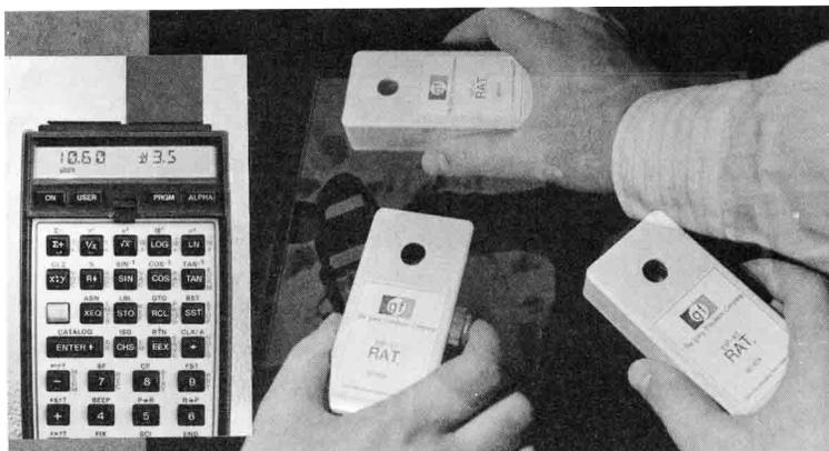
**Step 2** Using the RAT, take density readings of the brightest, darkest, and "18% grey-est" areas of your negative. The 41 will recommend a contrast filter and exposure time.
