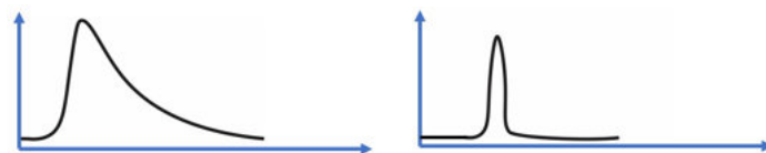
Typical flash output at full setting (left) and 1/16 th (right). The timing at the fastest focal plane shutter sync speed is just before the rise in output so always gets most of the duration – but precise timing adjustment in microseconds is needed for very fast global shutter speeds to match the peak output.
