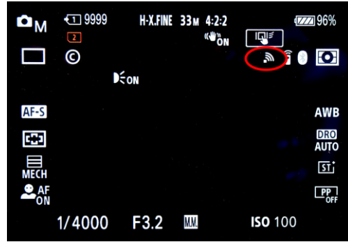
Figure 10: The new icon showing Wi-Fi signal strength when connected. (Red circle)
