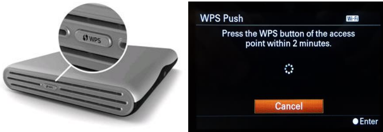
Figure 2-9: Many modern Wi-Fi routers possess a WPS button to make the setup of secure networks a push-button affair (left). Just push the button and then initiate “WPS Push” from the camera (right).
